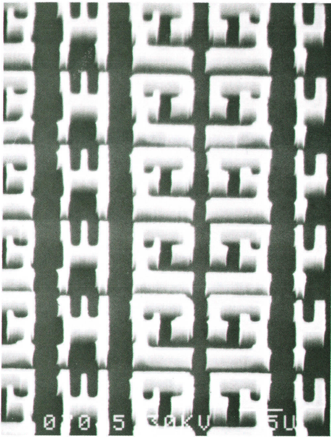
Fig. 9. This is a scanning electron micrograph of the isolation level for a portion of a random-access memory (RAM) patterned in the bottom layer of a trilevel resist structure. The top layer was exposed in the HP electron beam lithography system. The multilayer process reduces proximity effect and gives high-aspect-ratio lines ideal for masking dry etch processes. The smallest critical dimensions shown are 1\ \mu\text{m} .
